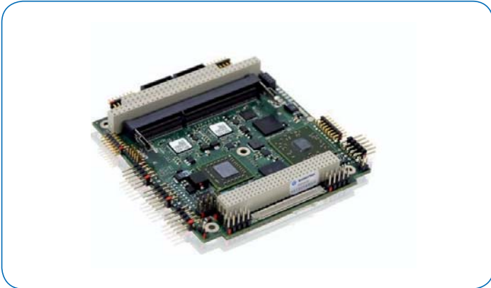
The Kontron PC/104-plus single board computer MICROSPACE® MSM-eO(-N) with the AMD Embedded G-Series APU features full ISA support.
