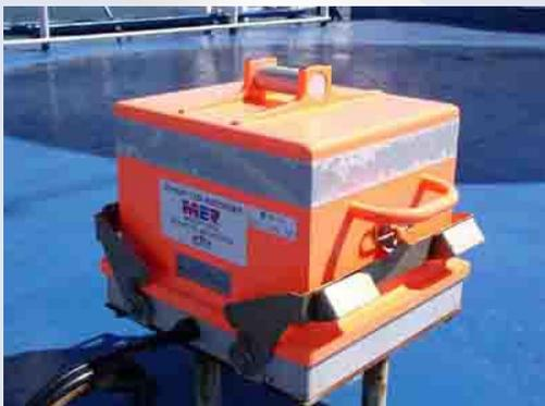
them for more than 12 hours. For example, a special rule algorithm stops the recording at the time of a collision so that the crucial event window remains documented. Thus, the stored data offers the basis for a realistic and objective evaluation.
