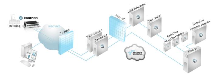
// The Wattics Sentinel energy monitoring gateway based on Kontron's Industrial Computer Platforms KBox-A101 is the central 'edge node' at the customer's site. It is connected to both the local energy grid as well as to the Sentinel grid built on modern IoT technologies.
