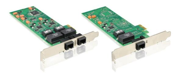
**Eching, Germany, June 01, 2010** – Today Kontron announced the <u>PCIe Medical LAN Card</u>, an IEC60601-1 compliant PCIe Gigabit Ethernet card, which can be used for the direct network connection of conventional IT equipment to medical devices. With this card, expensive medical LAN isolators, which otherwise would have to be inserted between the LAN port and a medical device, are no longer needed lowering costs and simplifying overall system design
