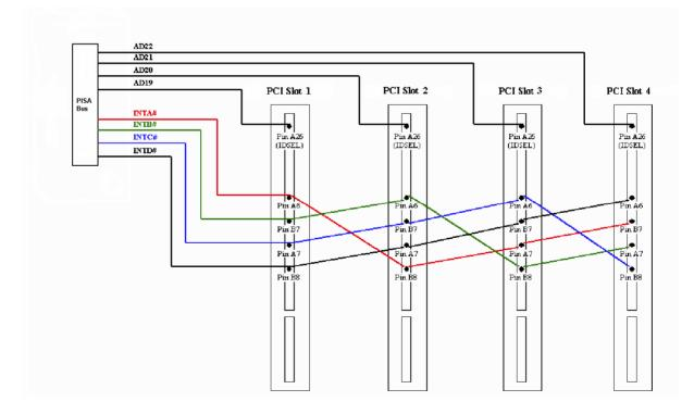
Attension: There are CPU boards and backplanes on the market designed as PCISA. These boards have a different PCI interrupt routing not following the PCI 2.1 recommendations. Check with your supplier, whether the boards you intend to use are PISA compliant or following PCISA standard.
