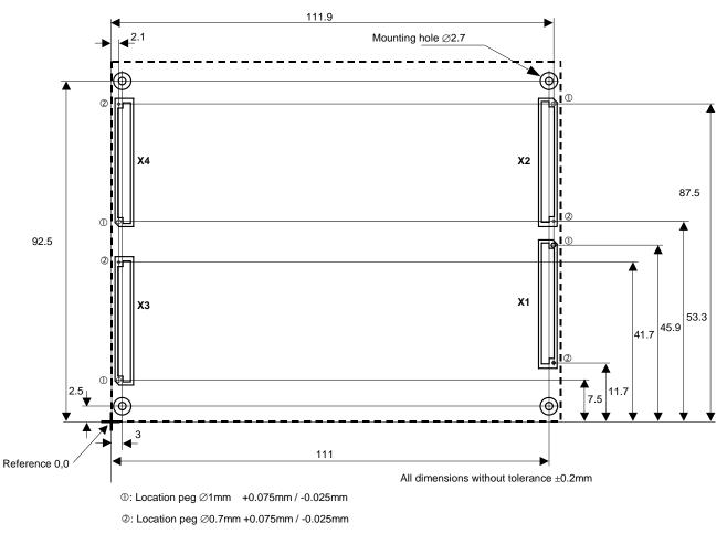
The outline shown here is for modules with a Y dimension of 95mm. To accommodate both 95mm and 100mm ETX modules, the 95mm outline shown here should be expanded by 2.5mm on the top and 2.5mm on the bottom.
