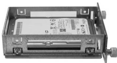
Fig. 25: Removed HDD tray with installed HDD (SATA0)
