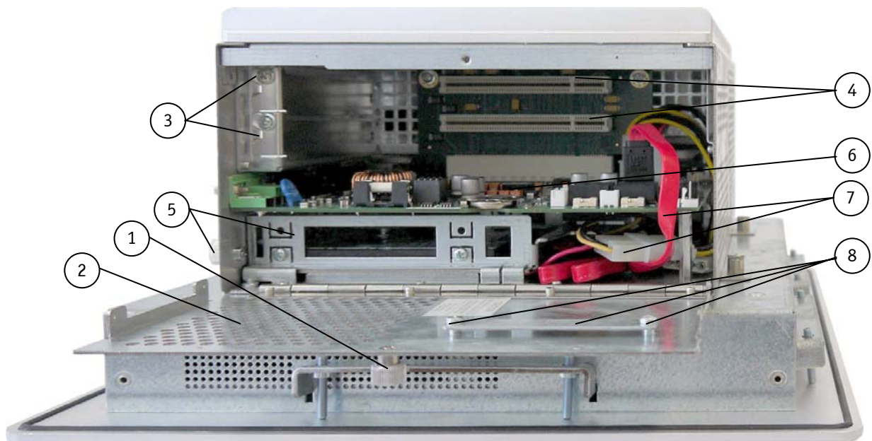
Fig. 19: V Panel Express system – opened access door (systemis shown with PCI expansion slots)
