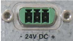
Fig. 9: Detail of the DC Power connector shown without Phoenix terminal
