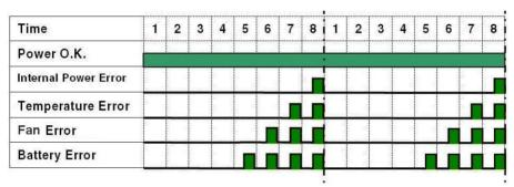
Fig. 11: Power LEDs and Error Codes
