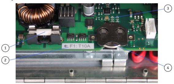
Fig. 17: Fuse, label for fuse value and Lithium battery location
