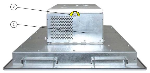
Fig. 18: Open the access door of the V Panel Express System
