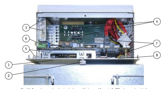
Fig. 19: Opened access door (systemis shown with riser card for up to 2x PCIe x1 expansion slots)
