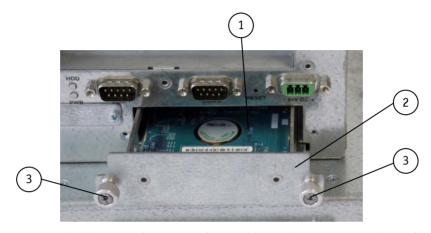
Fig. 12: Detail with drive tray for SATA HDD (shown with opened removable HDD drive tray)
