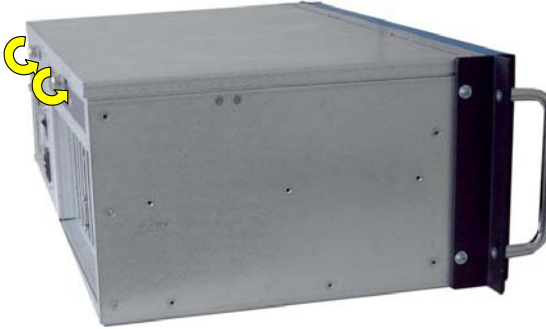
Fig. 19: Loosen the captive knurled screws
