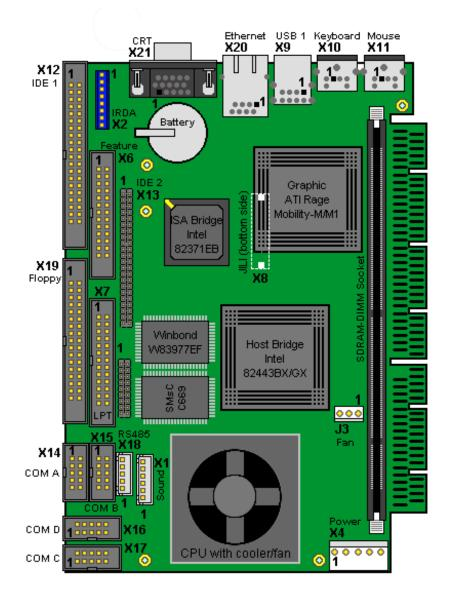
**Notes**: The position of Pin 1 is marked with a quadratic pad on the PCB.
