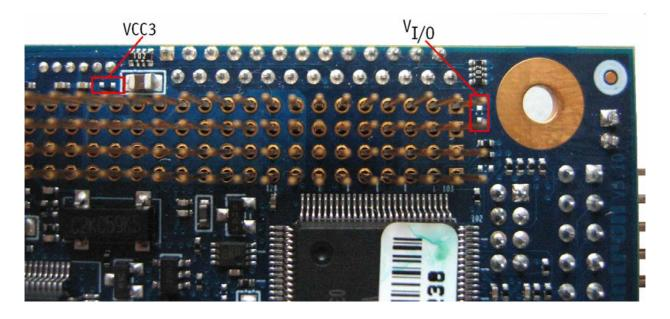
Attention: 5V PCI expansion cards can damage the board. Please note that the +5V supply voltage is routed to the connector. Four slots are available via the connector X11000 (IDSEL, /IRQ) but only three slots are busmaster capable.
