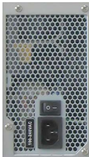
Fig. 19: Detail: 650W AC wide range PSU
