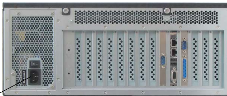
Fig. 36: KISS 4U V2, rear side without PE marked grounding stud
