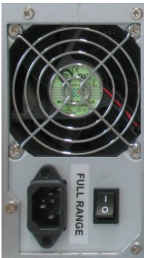
Fig. 18: Detail: 400W AC wide range PSU
