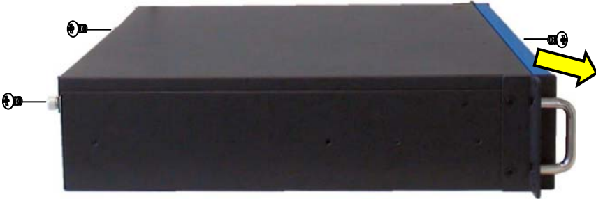
Fig. 13: Loosening the knurled screws which secure the cover
