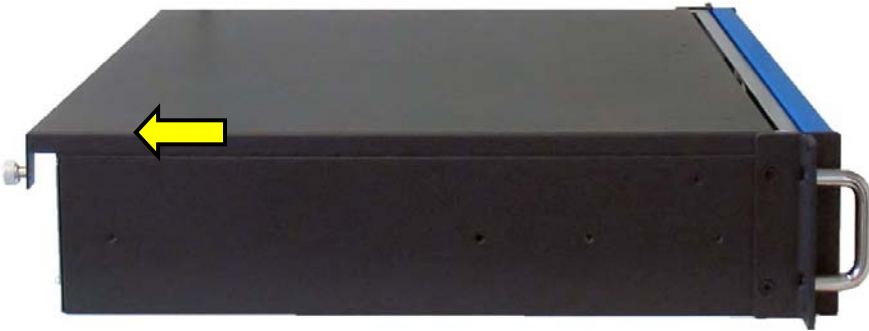
Fig. 14: Sliding back the cover will pull out the cover fixing brackets from the retaining brackets of the chassis.
