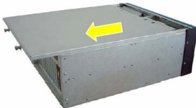
Figure 16: Removing the device cover
