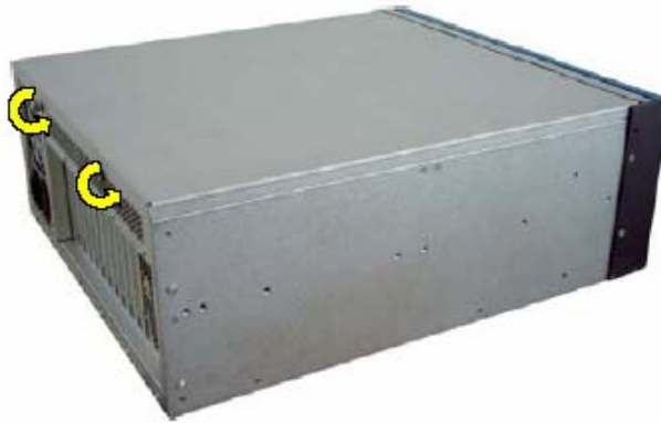
Figure 15: Loosen the captive knurled screws
