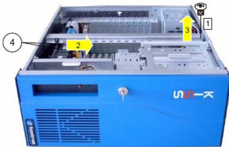
Figure 18: Removing the fastening screw the card hold-down bracket
