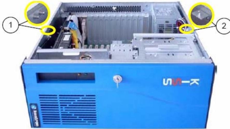
Figure 19: Bolts and fastening point for the card hold-down bracket
