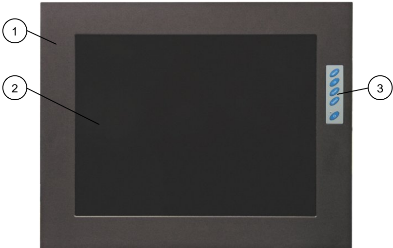
Fig. 2: KFM21_e – with front side mounted operating elements and LED indicator)
