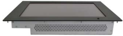
Fig. 8: Air openings (bottom side)
