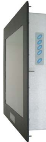
Fig. 3a: KFM_19e – Laterally installed controls
