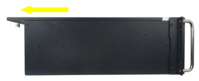
4. Lift the cover up (on the rear edge) and remove the cover as shown in Figure 25.
