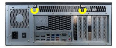
3. Pull the cover out slightly as shown in Figure 24 to release the cover's centering and fixing brackets (Figure 20, pos. 3 and pos. 4) from the retaining brackets of the chassis (Figure 21, pos. 4).
