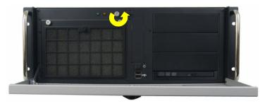
Figure 23: Loosening Knurled Screws (rear panel)
