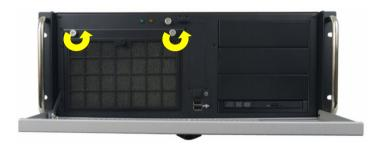
Figure 46: Fan Compartment (without fan assembly)
