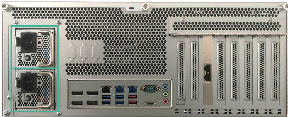
Figure 33: Redundant PSU Replacement
