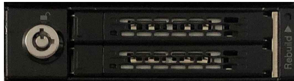
Figure 7: Dual 2.5" SSD Drive Mobile Rack (removable drives)
