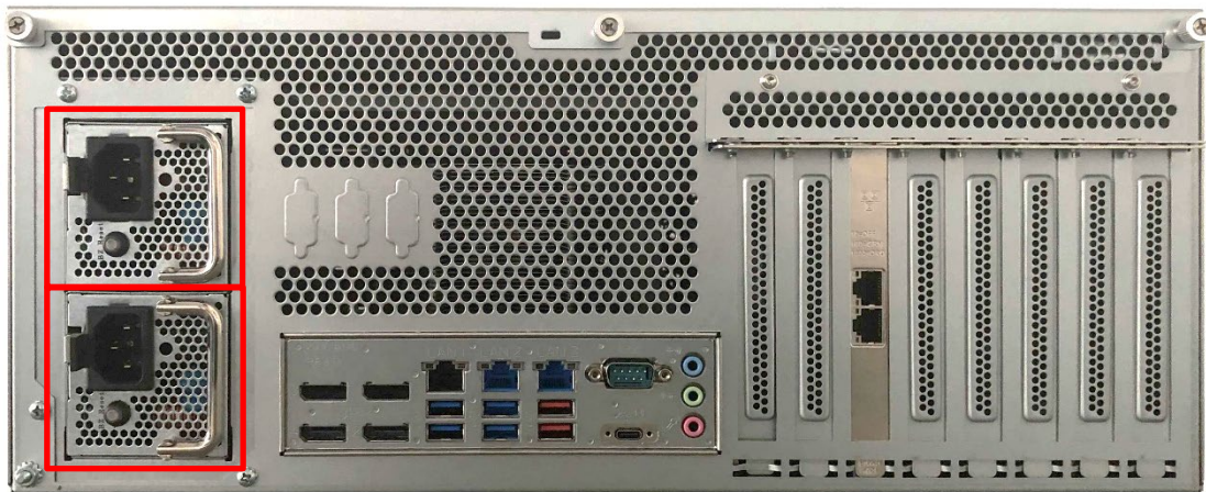
Figure 33: Redundant PSU Replacement
