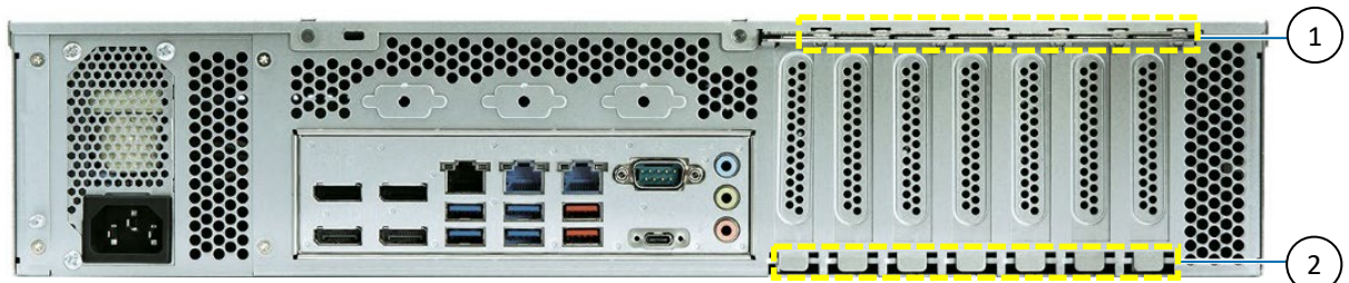
Figure 19: Installing Low Profile Expansion Cards
