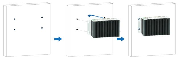
The front I/O panel can be placed downward depending on usage requirements, application scenarios and / or surrounding conditions.
