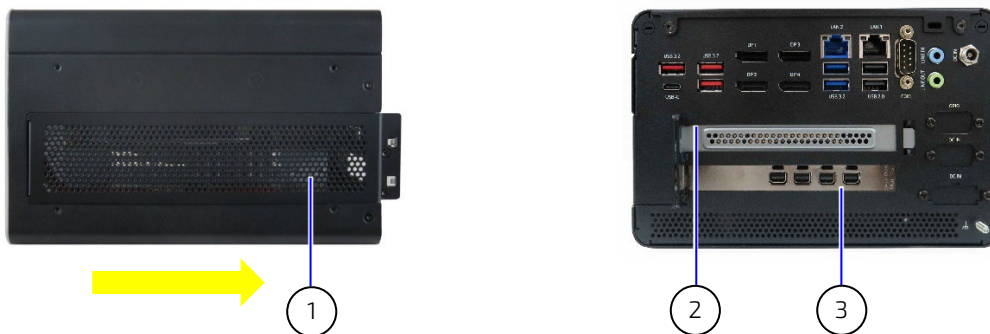
Figure 15: Removing Expansion Door
