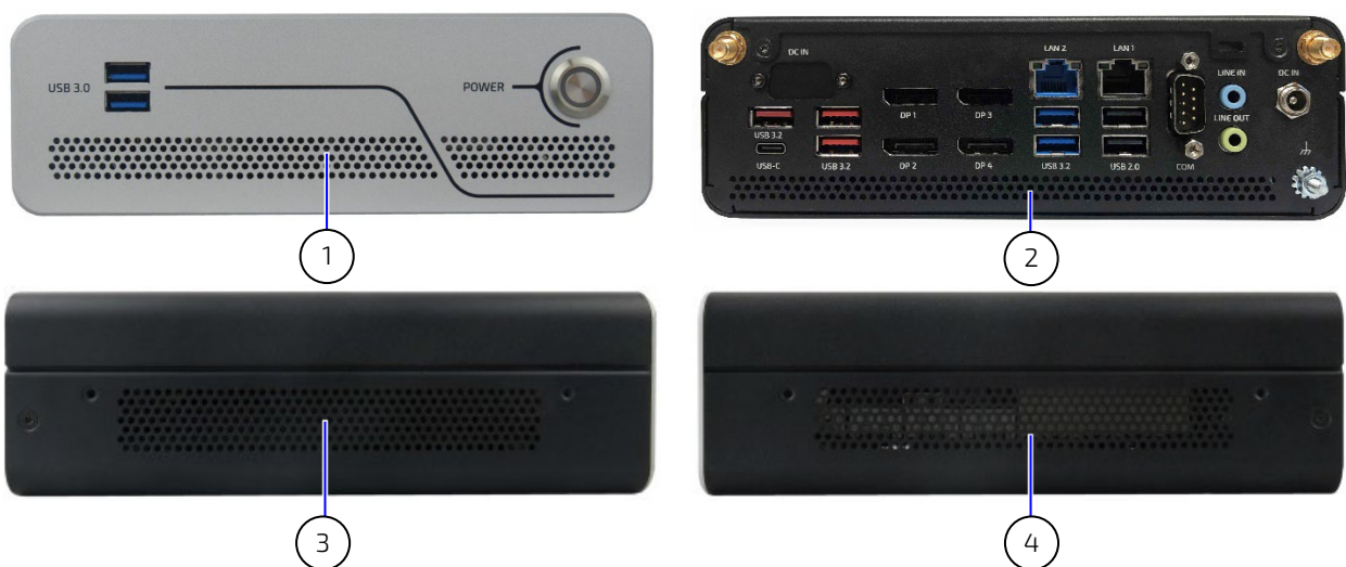
Figure 10: Ventilation Openings (output)
