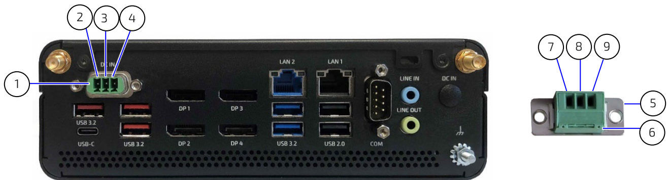
Figure 34: DC IN 3-pin Power Connector and 3-pin Mating Power Connector
