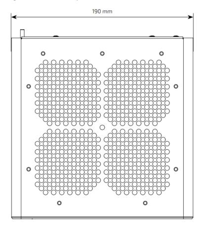
Figure 41: Dimensions Bottom Side
