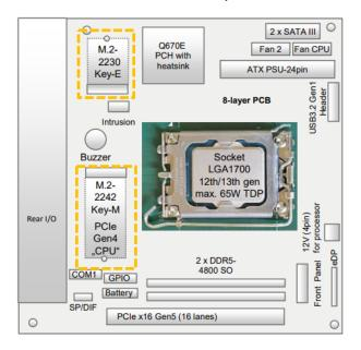
3. Insert the M.2 module into the corresponding M.2 socket gently and at an angle, until the hole on the M.2 module aligns with the corresponding motherboard's nut.
