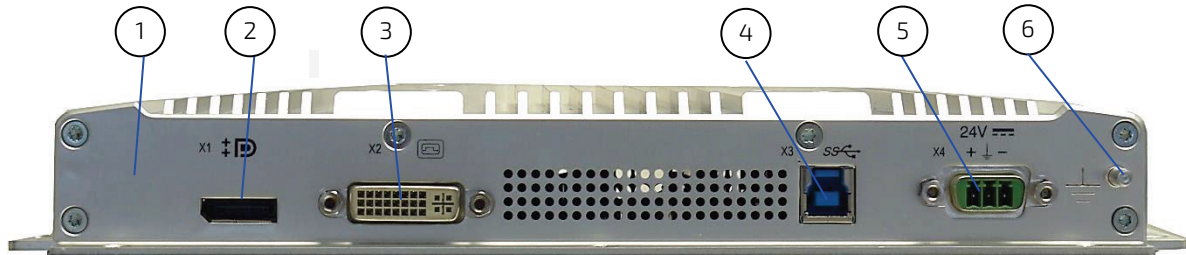
Figure 23: Bottom side of the FusionView (interface side of a 21.5" display)
