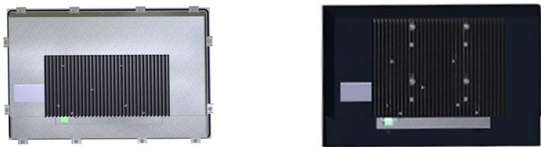
Figure 8: Rear Panel (panel mount and VESA) with Heatsink
