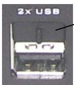
Fig. 13: Covered USB port for system configuration with equipped COM3 port
