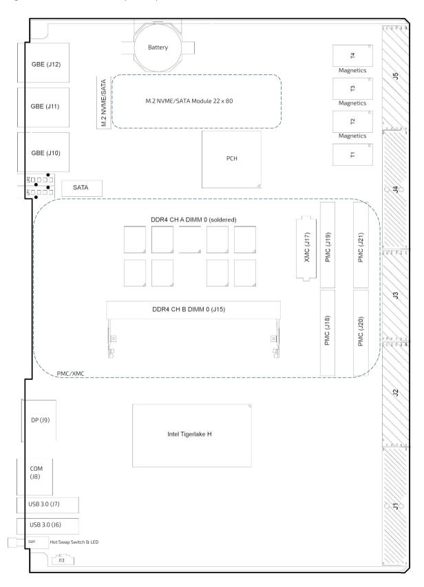
Figure 4: 4 HP CP6007 Board Layout (Bottom View)
