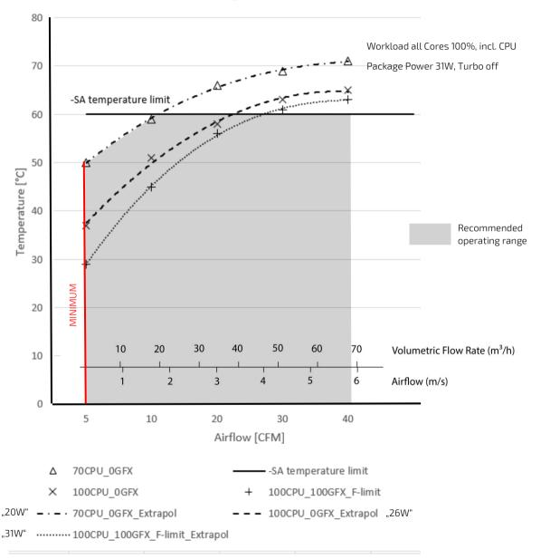
Figure 10: Ambient Temperature for Xeon® W-11555MRE, measured by Intel PTU Tool for Broadwell-DE rev. 1.1
