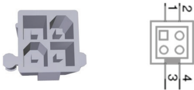
Figure 20: Internal Power Connector (J1)
