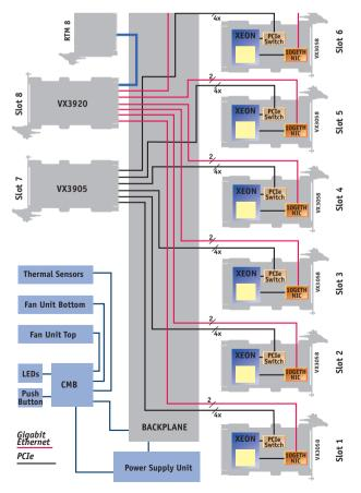
Kontron's sample turnkey system StarVX implements this architecture, targeting in maximum bandwidth. While computing power has been continuously increasing in the past, and I/O bandwidth did not, the balance of both is back again by Kontron StarVX.
