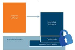
Software: Encryption of an application is performed by Kontron inside a dedicated security room by authorized personnel. Purchase of SEC-APPROTECT-INI allows for 10 encryptions service for the same project, allowing software updates this service includes the generation and delivery of the application key for one reference computer.
