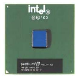
All Pentium®III or Celeron<sup>™</sup> processors in the innovative 370-pin FCPGA packaging giving a wide range of CPU speed can be used on the CP603. Active as well as passive cooling variants are available.
