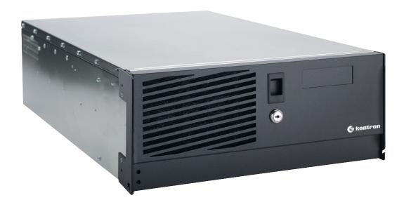
The 400-H33E is the latest PICMG1.2 4U platform. The 18-inch deep system comes standard with a rich set of features including the latest generation 478-pin processor technology, PCI-X support up to 133MHz, up to 4GB of DDR SDRAM, an onboard ATI® Mobility Radeon with integrated 16MB of DDR SDRAM and a dual Fast Ethernet controller.
