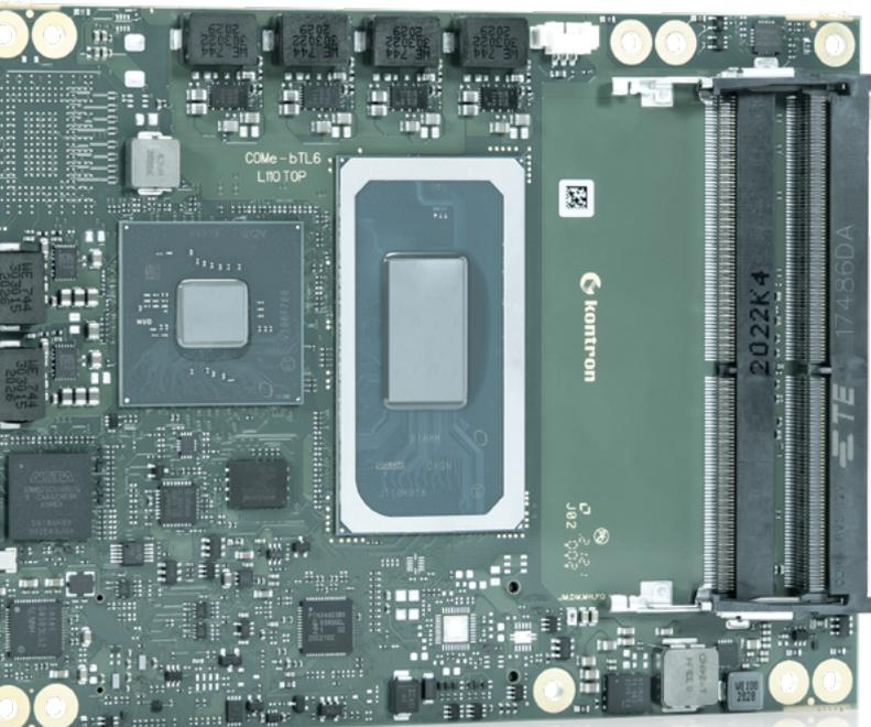
// 11th generation Intel® Core™ and Celeron® processors (previously known as Tiger Lake H) with up to eight cores provide COM Express® modules of the Basic form factor with the ability to perform high-end applications requiring a high bandwidth.
