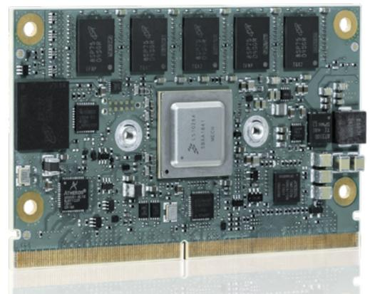
// Up to five integrated TSN-ready 1 GByte Ethernet ports, an integrated TSN switch and an NXP Dual Arm® Cortex®-A72 LS1028 processor as well as a 3D GPU make the SMARC-sAL28 module the perfect choice for use in IIoT or Industry 4.0 systems. It comes in the SMARC™ short-size form factor and is certified for the -40 °C to +85 °C industrial temperature range.
