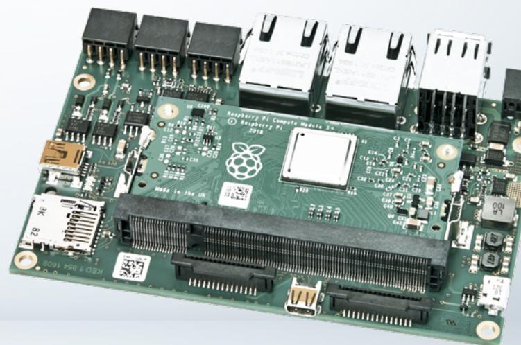
// An industry-grade variant of Raspberry Pi, Pi-Tron CM3+ features a CANbus interface and was extended by the CODESYS environment for application software development according to IEC 61131-3. This makes the compact board a prime choice for industrial control equipment.
