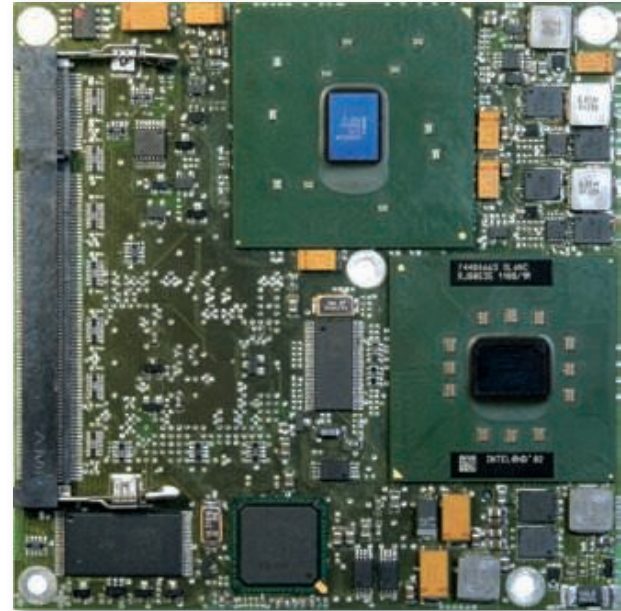
The ETXexpress-CD with IntelCore 2 Duo ist he latest high-end COM and was first introduced on the Embedded World 2007.
