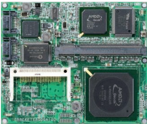
ETX-LX 3.0: The ETX-LX is the first COM applying to the ETX 3.0 specification with SATA on board and 100 percent pin-to-pin compatible to previous ETX base board designs.
