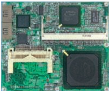
ETX-LX 3.0: The ETX-LX is the first board from Kontron built in accordance with the ETX 3.0 Specification, with SATA on board and 100 percent pin-to-pin compatibility with previous ETX Baseboard Designs
