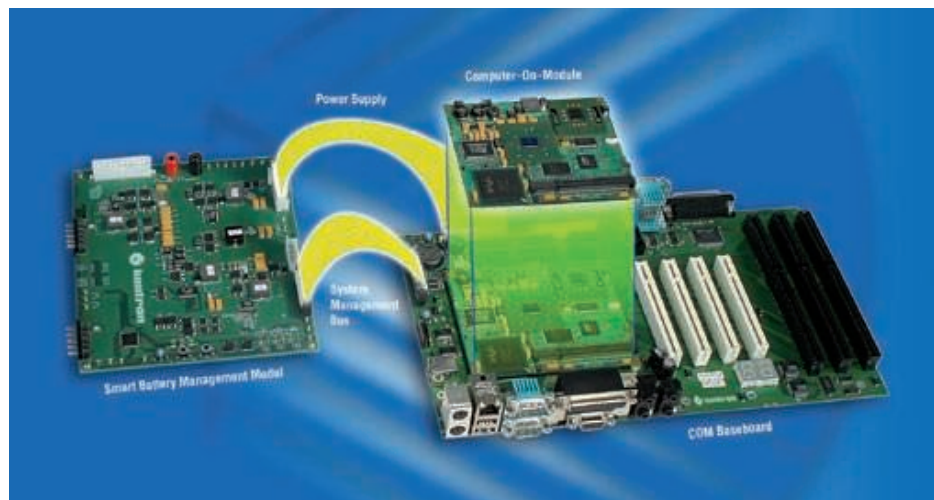
The evaluation board for MARS integrates the four reference designs SMART Battery System, Input Buck Boost Converter, Dual Buck Converter and Buck Boost Converter. Their layout files can be integrated into the custom baseboard layout simply by “copy & paste”
