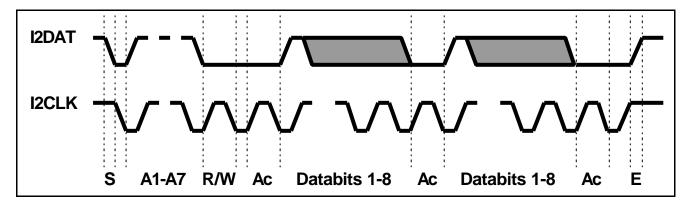
After the start condition (S) the slave address byte is sent. This byte consists of seven address bits (A1-A7) and one direction bit (R/W) with low level indicating a transmission (WRITE) and high level indicating a request for data (READ).
