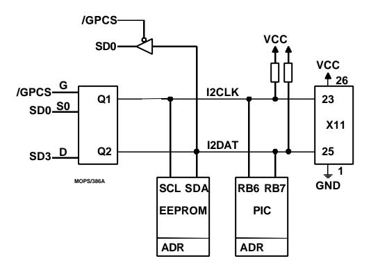
The signal line SD0 selects the I2CLK or I2DAT line for output. The signal line SD3 holds the "data", when set to 0 the selected line I2CLK or I2DAT is pulled LOW.
