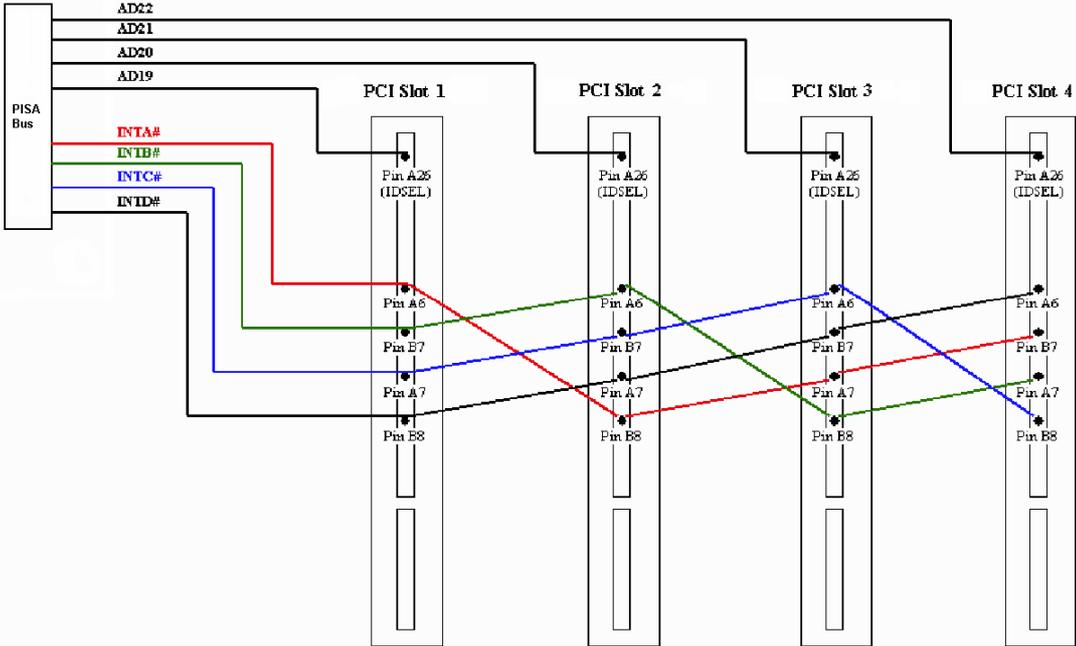
**Attention:** There are CPU boards and backplanes on the market designed as PCISA. These boards have a different PCI interrupt routing not following the PCI 2.1 recommendations. Check with your supplier, whether the boards you intend to use are PISA compliant or following PCISA standard.
