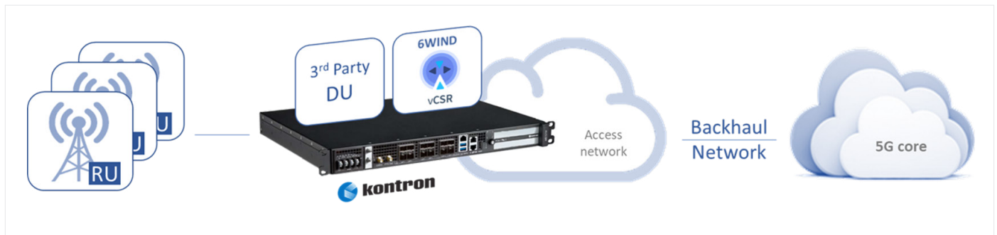
Figure 2. 6WIND virtual cell site router in a typical cell site.
