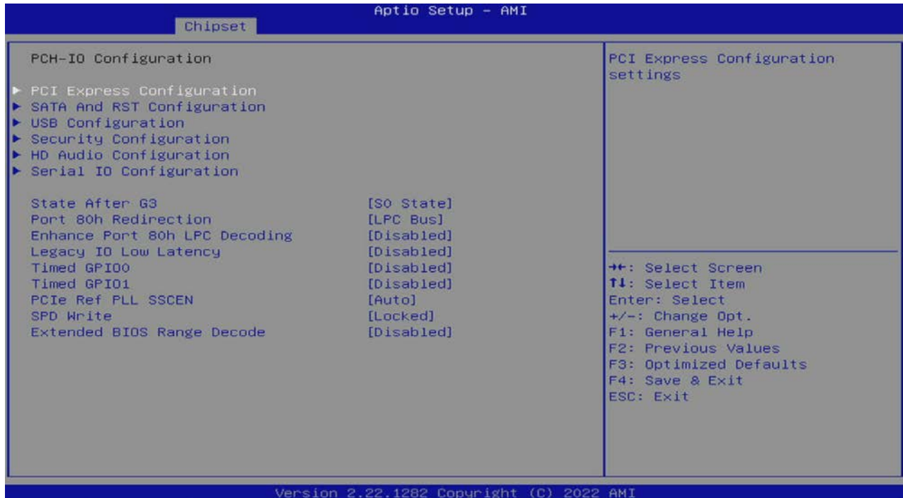
Figure 19: Chipset PCH-IO Configuration Setup menu Initial Screen
