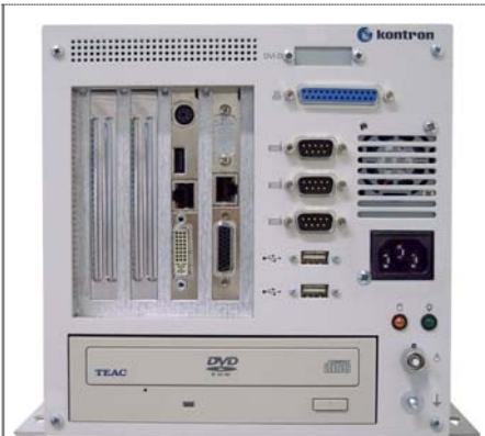
Fig. 3: SC-75_e with P7 SBC (AC version)
