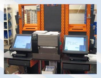
The individual terminals are not equipped with a memory of their own, but are controlled by the central processor through a constant connection via Ethernet and PXE boot.
